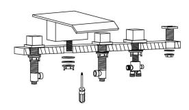
6. Pulling pipe connect with the connector A through the shower holder. Gravity ball fixed on the top of the pull out pipe. Water nozzle connect to the conversion B, hot and cold switch connect with connector C and D respectively and finally contact to the hot and cold water hose.
