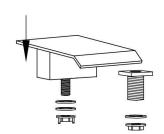
4. Three switches main body from the bottom up through the table, fasten the screw and handle by hexagonal tool after alignment to the base. Finally fasten the nut.
