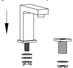
4. Three switches main body from the bottom up through the table, fasten the screw and handle by hexagonal tool after alignment to the base. Finally fasten the nut.
