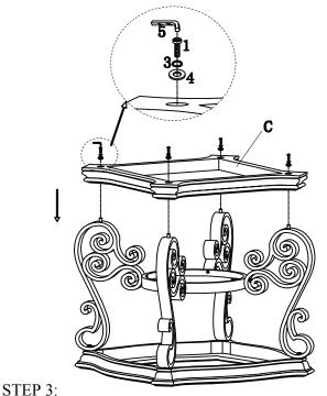
Attach Bottom Panel (C) to Legs (E) by using Allen Key M4 (5), Allen Bolt 1/4"x 50mm (1), Spring Washer 1/4"(3), Flat Washer 1/4"(4)
