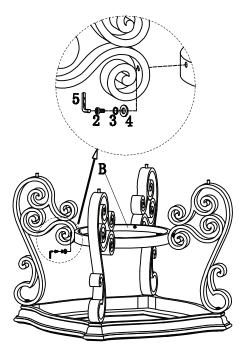
STEP 2: Attach Shelf (B) to Legs (E) by using Allen Key M4 (5), Allen Bolt 1/4" x1"28mm (2), Spring Washer 1/4" (3), Flat Washer 1/4" (4)
