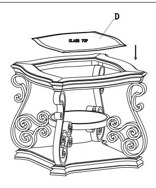
STEP 4: Turn over the table. Tighten all bolts carefully and Insert Glass top (D) into the Top Frame (A)
