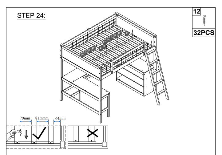
Note: Do not lock the screws of the bed slats to the outermost edge of the bed slats, you need to leave a certain space at the edges, otherwise it will cause the board to break. Do not lock the bed slats on the edge of the wood, please hold firmly before screwing, hold it in place with one hand, then lock the screw.
