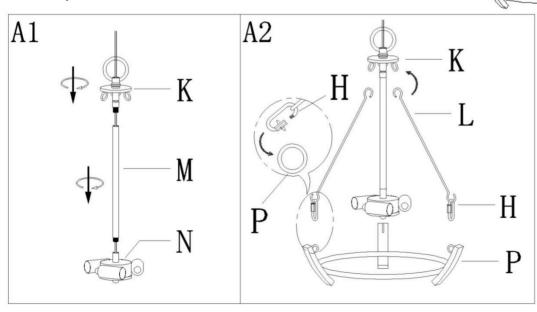
Step A1: Pass fixture wires through stem (M) and fixture loop assembly (K).
