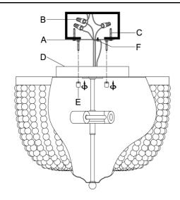
**Step 5:** Attach the Lamp Body(D) to the junction box and fix it by turning the Canopy Nut(E) clockwise.
