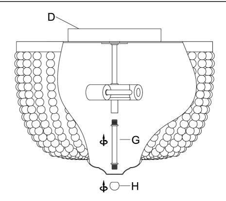
**Step 2**:Fix one end of Tube(G) to the Lamp Body(D) in a clockwise direction, Place the iron frame below the Lamp Body (D) on the threaded part of the Tube (G). The iron frame at the bottom of the lamp body is shown in the figure. Turn the Finial (H) clockwise until tight.
