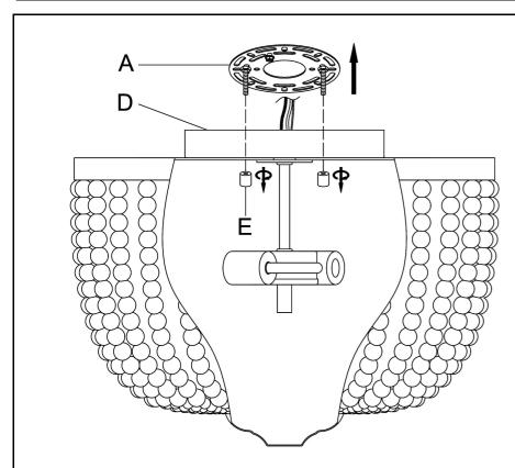
**Step 1**: Unpack all parts from cartons carefully. Turn the Canopy Nut (E) counterclockwise to separate the Mounting Plate (A) and Lamp Body (D).
