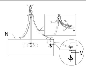
**Step 3:** Adjust the angle of the spider of the Lamp Body (L). Insert the portion of each spider into the top hollow of the Shade (N), then fix them with Ball Nut (M), tuning each Ball Nut (M) clockwise till tight.
