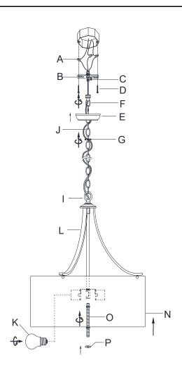
**Step 5:** Attach the Mounting Plate (B) onto the junction box with two Mounting Screws (D). Slide the Canopy (E) upward along the chain(J) till the ceiling surface. Fix it by rotating the Canopy Nut(G) clockwise to engage it with the threaded portion of the Hanging Loop (F) until secure. Do not over tighten this nut. Insert the bulbs (K) into the sockets until secure.
