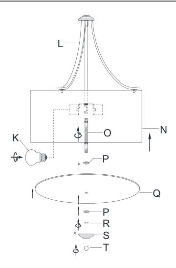
**Step 6:**Screw the Threaded Stem(O) into the tube underneath of the socket assembly as diagram. Place the Plastic washer (P) onto the Threaded Stem(O) then the Diffuser (Q) ,Plastic washer (P). Fix them with Hex Nut (R).Attach the Metal Cover (S), fix it with Finial (T).
