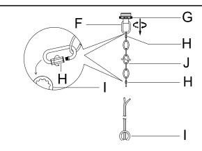
**Step 1:**Unpack all parts from cartons carefully. Screw the Chain(J) to the Hanging Loop(F) and the Fixture Loop (I) with Closable link/cap (H) as diagram.
