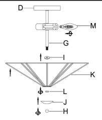
**Step 6:** Insert the Bulbs (M) into the Sockets as diagram. Set the middle hole of the Gasket (I) and Shade (K) into the threaded part of the Tube (G), turn the Nut (L) clockwise to be tightened, then set the Cover (J) into the threaded part of the Tube (G), turn the Finial (H) until tightened.
