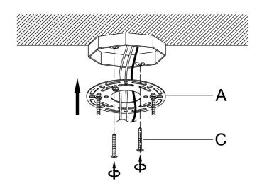
**Step 4:** Fix the Mounting Plate(A) to the junction box with Mounting Screw (C).
