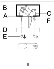
**Step 5:** Attach the Lamp Body(D) to the junction box and fix it by turning the Canopy Nut(E) clockwise.
