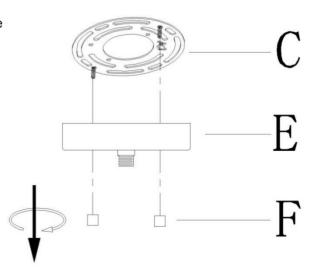
3 » Pass the fixture wires through tube (G) and canopy (E), then screw tube (G) onto canopy (E) and the top of sockets assembly (K).
