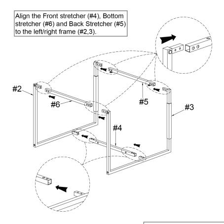
Secure by using Bolts (#A) with Washers (#C).
