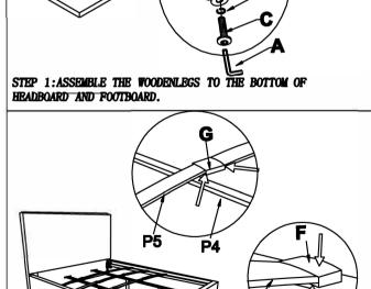
STEP 4: INSERT CLIPS (F) TO SIDE RAILS' TUBE. INSERT SLATS | STEP 5: INSERT CLIPS (G) INTO THE MIDDLE TUBES OF THE TO THE CLIPS (F). THEN CONNECT THE TWO SIDE'S OF THE SLATS REMAINING SLATS TO THE BED FOUNDATION. TOGETHER BY CLIPS (G).
