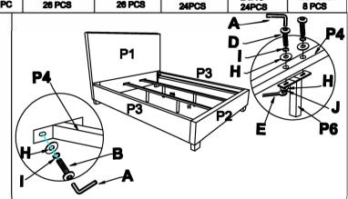
STEP 3: CONNECT THE METAL TUBE TO THE HEADBOARD & FOOTBOARD WITH BOLT (B) BY WRENCH (A). ASSEMBLE THE SUPPORT LEG (H) TO THE BOTTOM OF TUBE WITH BOLT (D) BY WRENCH (A).
