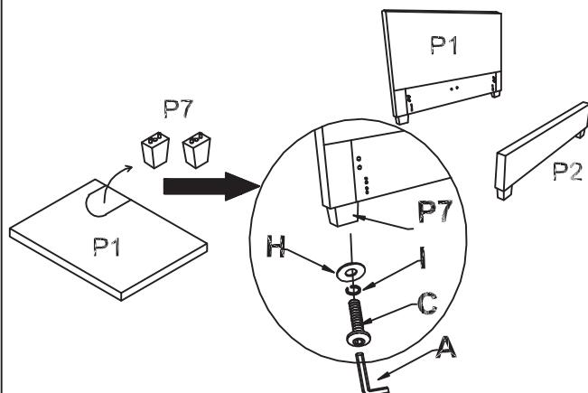
STEP 1: ASSEMBLE THE WOODEN LEGS TO THE BOTTOM OF HEADBOARD AND FOOTBOARD.
