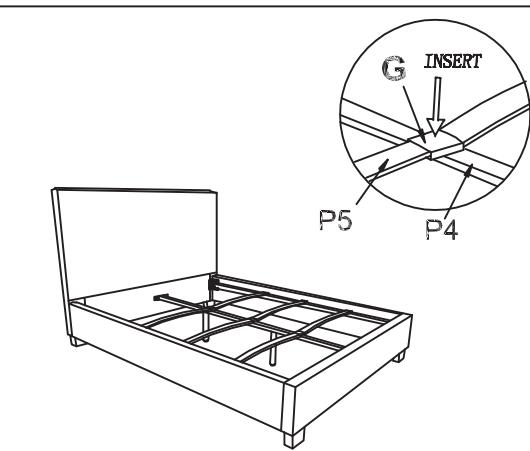
STEP 5: INSERT CLIPS (G) INTO THE MIDDLE TUBE OF THE REMAINING SLATS TO THE BED FOUNDATION.
