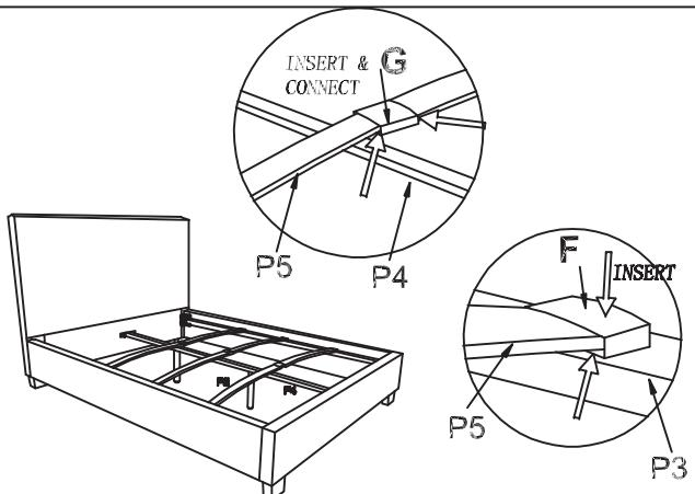
STEP 4: INSERT CLIPS (F) TO SIDE RAILS' TUBE. INSERT SLATS TO THE CLIPS (F), THEN CONNECT THE TWO SIDE'S OF THE SLATS TOGETHER BY CLIPS (G).
