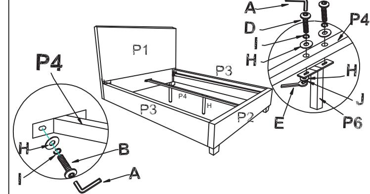
STEP 3: CONNECT THE METAL TUBE TO THE HEADBOARD & FOOTBOARD WITH BOLT (B) BY WRENCH (A). ASSEMBLE THE SUPPORT LEG (H) TO THE BOTTOM OF TUBE WITH BOLT (D) BY WRENCH (A).
