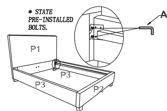
STEP 2: LOOSEN THE BOLTS OF HEADBOARD (P1) & FOOTBOARD (P2). CONNECT THE SIDERAIL (P3) WITH HEADBOARD (P1) AND FOOTBOARD (P2) BY HOOK, TIGHTEN THE PRE-INSTALLED BOLTS BY WRENCH (A).
