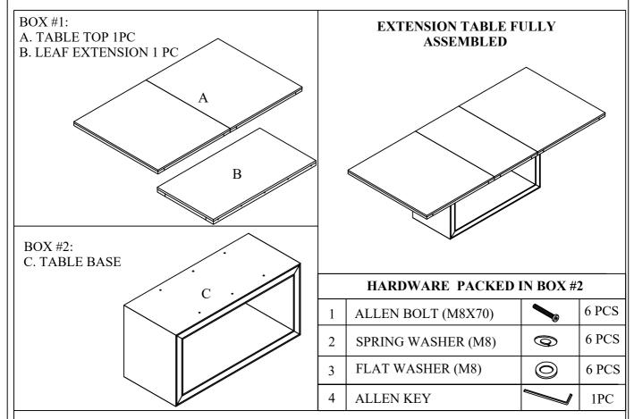
STEP 1: ATTACH TABLE TOP (A) TO THE TABLE BASE (C) USING SIX ALLEN BOLTS (1), SPRING WASHERS (2) AND FLAT WASHERS (3). TIGHTEN COMPLETELY WITH THE PROVIDED ALLEN KEY (4). WASHER (3), SPRING WASHER (2), ALLEN BOLT (1) AND SECURE WITH ALLEN KEY (4).
