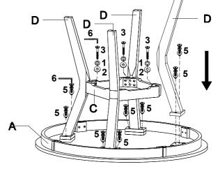
Don't tighten the bolts untill last step
