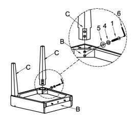
DO NOT TIGHTEN BOLTS COMPLETELY
