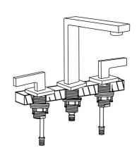
4. Connect the pipe of spout and two handles
