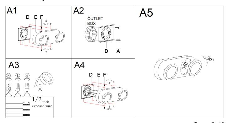
Step A1 » Unscrew screws (F) from back plate (E), then set them aside for later installation.
