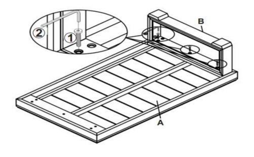
With assistance from your adult partners, turn the Table Top (A) (bottom-side up) and place on a clean, non-marring surface to avoid any scratches or damage to the product. Attach the Leg Frame (B) onto the Table Top(A) using Bolts (1) and the Allen Wrench(2).
