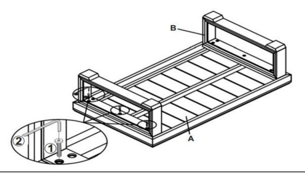
Attach the remaining Leg Frame (B) onto the Table Top(A) using Bolts (1) and the Allen Wrench (2)
