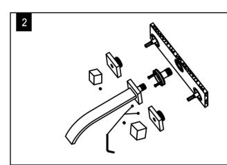
2. After installing the main valve body, the water to be tested is completed, and the pipeline and the main valve body can be covered after confirming that there is no leakage.
