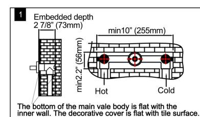
main valve body is 10"x2.2" and the depth is 2 7/8"(73mm).
