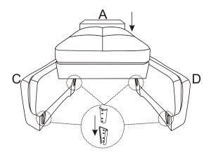
2 Attach Backrest (B) to Lsf Arm (C) and Rsf Arm (D) by using brackets as shown. Make sure brackets are secured in position.
