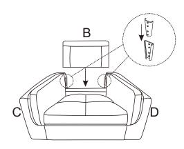
3 Insert Bolt (H) and Flat Washer (I) into the pre-drilled holes of Seat (A), Lsf Arm (C) and Rsf Arm (D) and tighten them.
