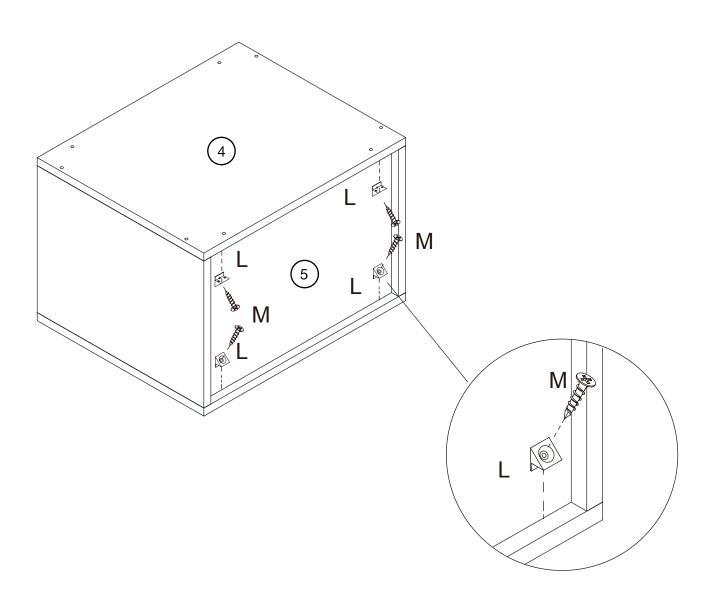
Remember that frame you put together in Step 1? Well, it's now ready to be put to use! Attach it to the Bottom Panel (4) and tighten to 100%.
