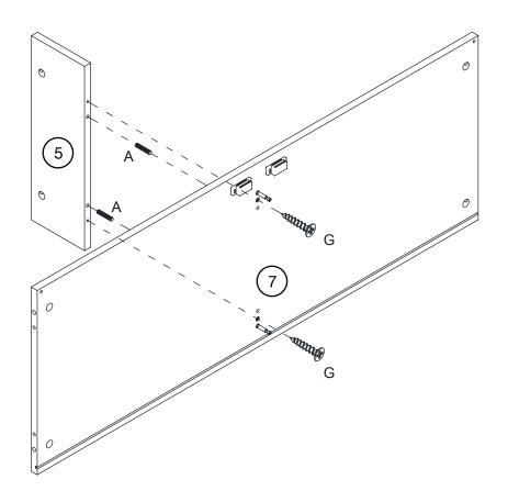
Attach the Bottom Divider Panel (6) to the Center Shelf (7). You're starting to get the hang of this!
