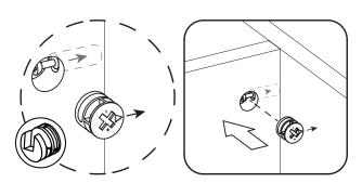
Using a screwdriver, you will turn the cam lock until it stops, usually between 130° or 180°. You will feel the panels pulling closer until they are secured.
