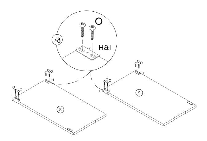
Take the doors and secure it to what you've built so far, being sure to line the Top Metal Hinge (I) with the corner hole on the unit. It's all coming together!
