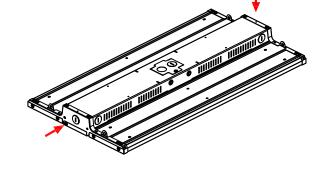
1. Screw out the nut and take out the gasket.
