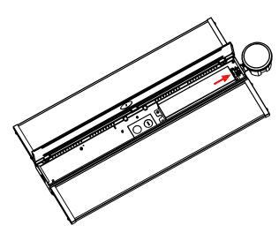
3. Open the junction box cover to the position shown in the figure (half open state), move away the knock-out, the microwave sensor go through the knock-out, fix the gasket, screwand tighten it.
