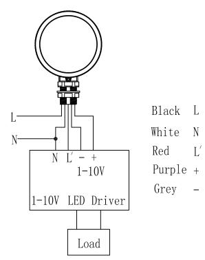
4. Wiring according to wiring diagram.
