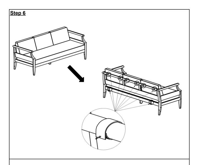
Connect the magic tape straps of the Back Cushions(E) and the Seat Cushion(F) to the Backrest Panel(D) and the Seat Panel(C) as shown in the above picture. Your 3 Seater Sofa is ready for use.
