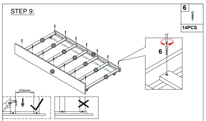
Note: Do not lock the screws of the bed slats to the outermost edge of the bed slats, you need to leave a certain space at the edges, otherwise it will cause the board to break.
