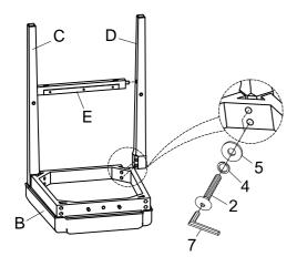
1.Loosely attach the Left leg(C) and Right leg(D) to the Linen Fabric Seat(B), using Bolts(7+2+4+5) to tighten, as shown.
