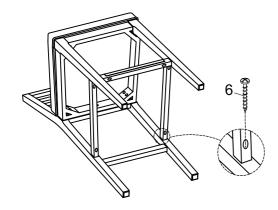
1.Attach the Front stretcher(E) and Right/Left stretcher(F/G) to the legs, using Screw(6) and a Philips head screwdriver to tighten, as shown.
