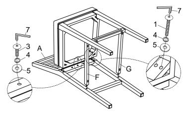
1.Loosely attach the Fabric Seat (B) to the Stool Back(A), using Bolts(7+3+4+5) and Bolts(7+1+4+5) to tighten, as shown.
