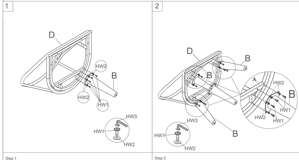
Attach Leg Chair (B) to Chair Seat Frame (D). Use Bolt (HW1) tighten with Allen Key (HW3).
