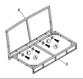
Step 1 Connect Bench back frame (5) & Bench seat frame (3), tighten Bolt (A) with Allen Key (D)
