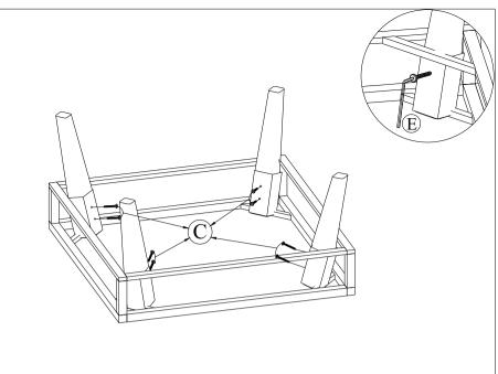
Step 2 : Connect The Part from Step 1 & tighten Screw Bolt (C), Flat Washer (D) with Allen Key (E).
