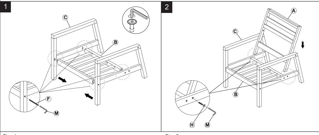
Step 1  $\label{eq:continuous} \mbox{Attach Frame Leg (C) to Frame Seat (B) ,use Screw (F) tighten with allen key (M). }$
