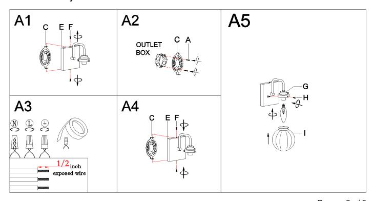
Step A1 » Unscrew studs (F) from back plate (E), then set them aside for later installation.
