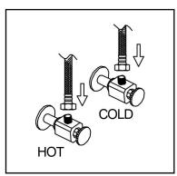
5. Attach flexible hose to water supply.
