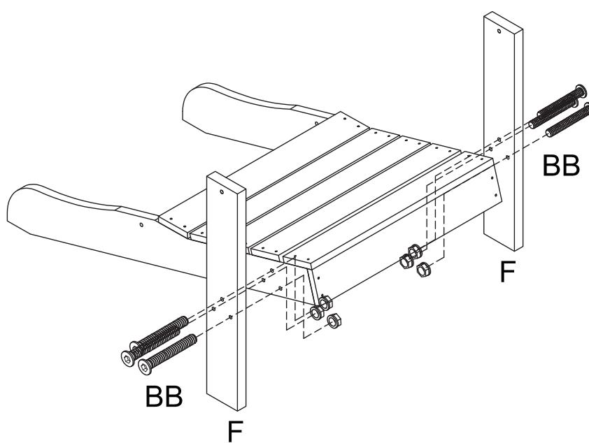
**\*Note: DO NOT TIGHTEN ANY BOLTS BEFORE THE UNIT PUT TOGETHER.**
