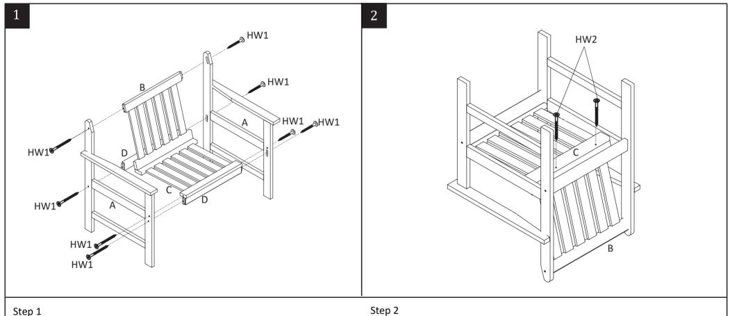
Use screws (HW1) to attach leg frames (A) to back frame (B), seat frame (C) & cross bar of leg (D), tighten with allen key (HW3).
