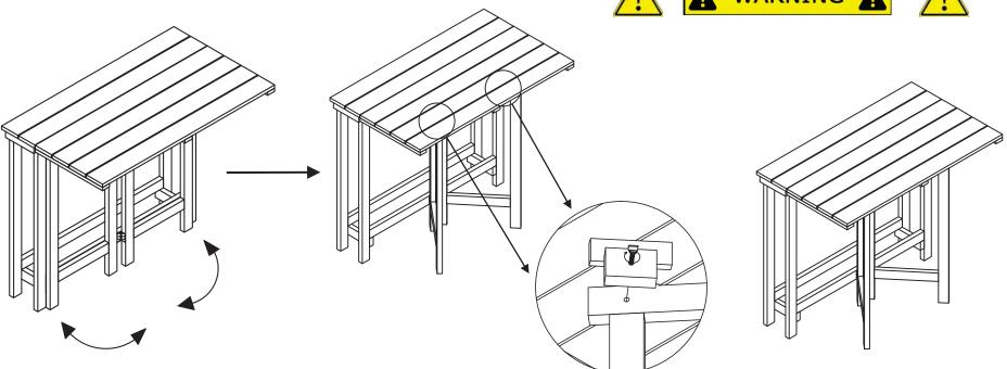
Lock the leg to the top by turn on the bolt to the hole as shown on the picture.
