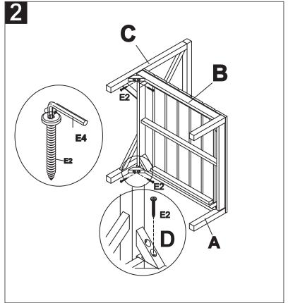
Step 1: attach the leg (A) and the back (C) to the seat (B) as shown on the picture. Then use the Allen Bolt (E1) and tighten it with the Allen Key (E4). Tighten the 2 legs (A) with the wrench(E5) as shown on the picture.
