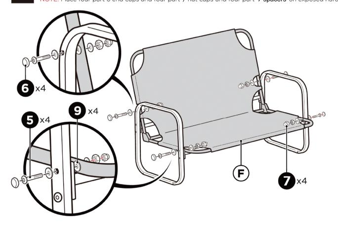
Attach the glider assembly to the seat sides with four part 4 bolt sets and four part 8 spacers. NOTE: Place four part 6 end caps and four part 7 nut caps on exposed hardware.
