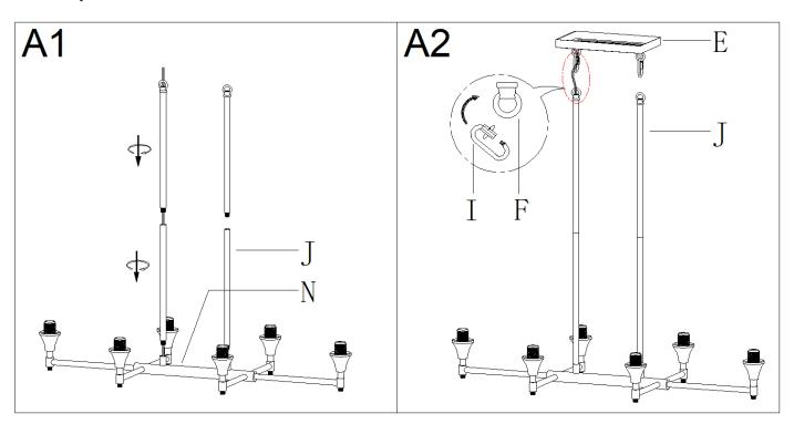
Step A1 » According to your desired hanging height to choose and use tubes (J). Then pass the fixture wires through the chosen tubes (J).
