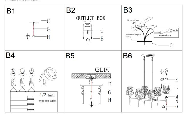
Step B1 » Unscrew hex nut (G) and cap nut (H) from single bar (C).
