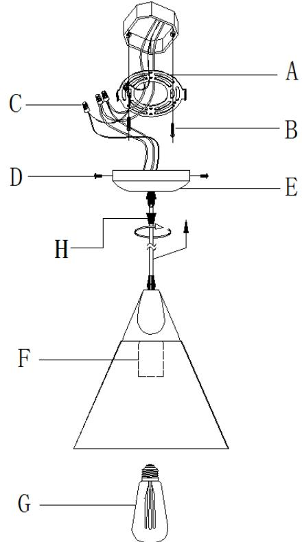
Loosen the screw(H) and push or pull the cord to adjust the cord length, then turn the screw(H) tightly to lock the cord after cord length adjusted finished.
