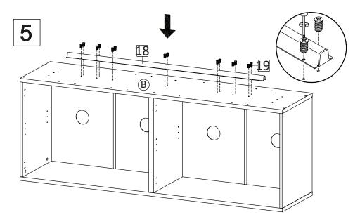
Place Anti Deflection Metal Bar (HW18), secure with screw M6.5x12,5 (HW19) using screwdriver.
