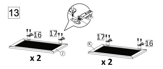
Insert Hinge (HW16) into pre-hole in Frame Door Left (J) and Frame Door Right (K). Secure with Screw M4.5 x 12.5 (HW17).
