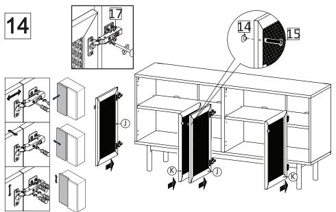
Install Frame Door Left (J) into Side Board Left and Center Board,
