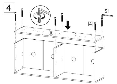
Put Bottom Board (B) and secure with Screw M7x50 (HW4), tighten screws using Allen Key (HW5)
