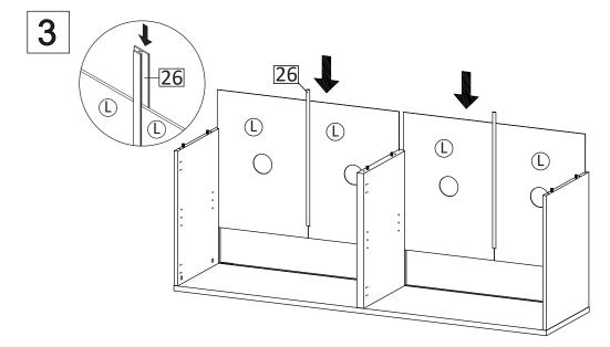
Insert Backboard (L) as figure and slide in the List Joint (HW26) in between two backboard.
