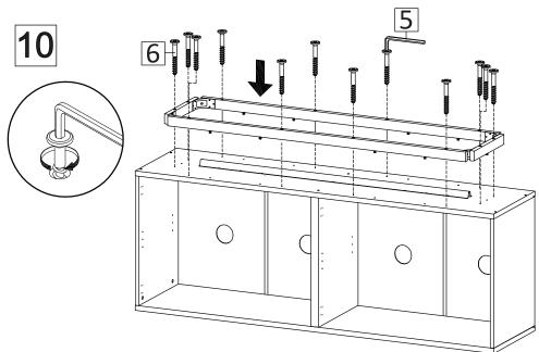
Bring the assembled bottom skirt and insert into Bottom Board of the cabinet. Secure with Screw M6.4 x 53 using Allen Key (HW5)
