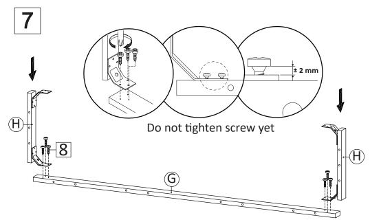
Combine the Bottom Skirt 2 from step 6 with Bottom skirt 1 (G), using Screw M4x16 (HW8). Do not overtight screw yet, leave around 2mm gap.
