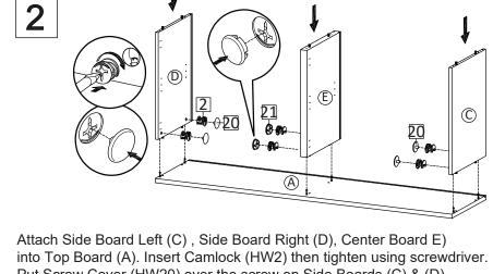
Put Screw Cover (HW20) over the screw on Side Boards (C) & (D), and put Screw Cap (HW21) over the screw on Center Board (E).
