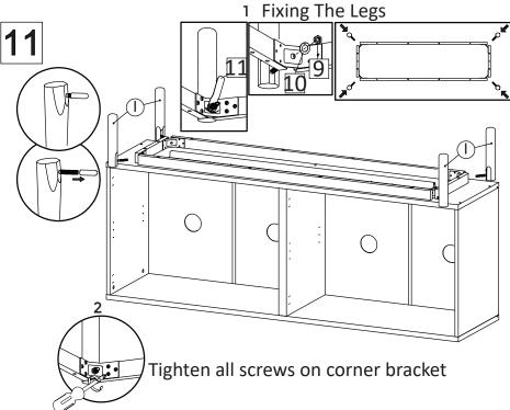
Remove plastic cap from Legs. Insert the bolt of the Leg (I) into hole of corner brace as shown in figure. Insert Spring Washer (HW10) first into the hanger bolt of leg, then followed by Nut (HW9), tighten all the nuts using provided Wrench (HW11). Ensure that all legs has been tightened,
