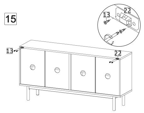
Attach Tip Protector (HW22) into back of Top Board using Screw M3.5x15.5.
