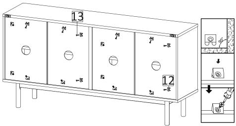
Use Wedge (HW12), Screw M 3.5 x15.5 (HW13) to tighten the back of media stand by using screwdriver.
