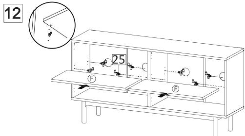
After bringing the product upright, insert Shelf Support (HW25) into the holes on Sideboard & Centerboard, on the desired level. Then place the Adjustable Shelf (F) by inserting the hole on the shelf into the shelf support
