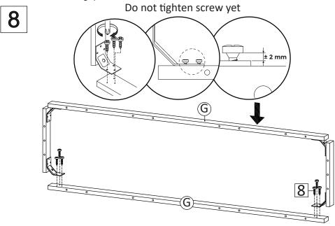
Combine components from step 7 with remaining Bottom skirt 1 (G), using Screw M4x16 (HW8). Do not overtight screw yet, leave around 2mm gap.
