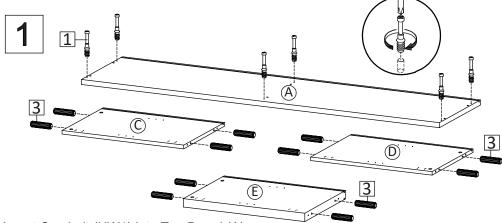
Insert Cambolt (HW1) into Top Board (A) Insert Dowel (HW3) into Center Board (E), Side Board Left (C) and Side Board Right (D)
