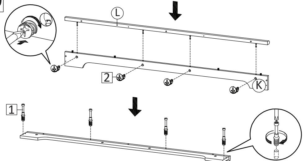
Attach Bottom Skirt 1 (K) and Bottom Skirt 2 (L) together by using Camlock (HW2) and screwdriver.
