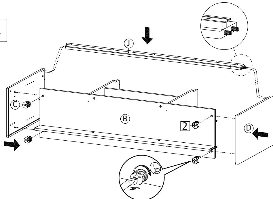
Combine step 4, step 7, Side Board Left (C) and Side Board Right (D) by using Camlock (HW2) and screwdriver.
