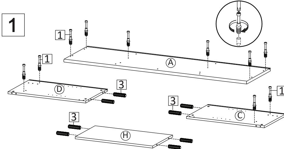
Insert Cambolt (HW1) into Top Board (A), Side Board Left (C) and Side Board Right (D).
