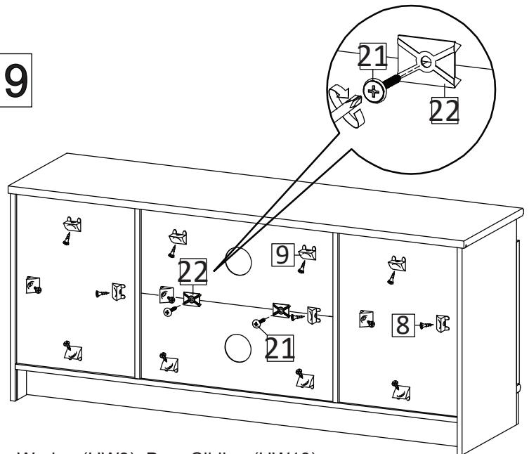
Use Wedge (HW9), Barn Sliding (HW10), Screw M 4x17 mm (HW21) and Back Panel Holder (HW22) to tighten the back of media stand by using screwdriver.
