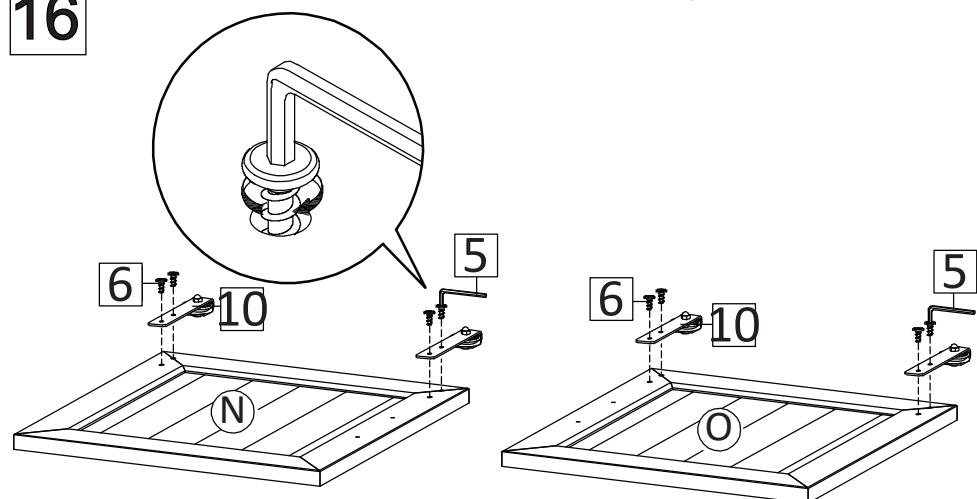
Attach Barn Sliding (HW10) to Frame Door Left (N) and Frame Door Right (O) by using Screw M 6.4x14 mm (HW6) and tighten them with Allen Key (HW5).
