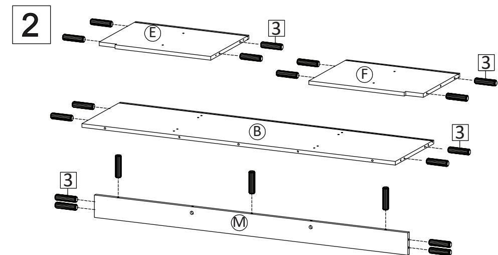
Insert Dowel Big (HW3) into Centre Board Left (E), Centre Board Right (F), Bottom Board (B) and Support Board (M).
