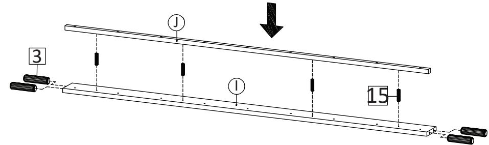
Put Front Skirt 1 (I) and Front Skirt 2 (J) together by using Dowel Big (HW3) and Dowel Small (HW15).
