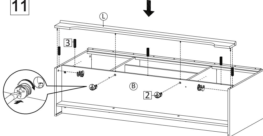
Put step 10 together with step 8 by using Camlock (HW2) and screwdriver.
