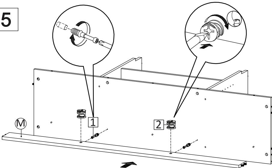
Insert Cambolt (HW1) into Camlock (HW2), tighten Camlock (HW2) using screwdriver to attach Support Board (M) to step 4.
