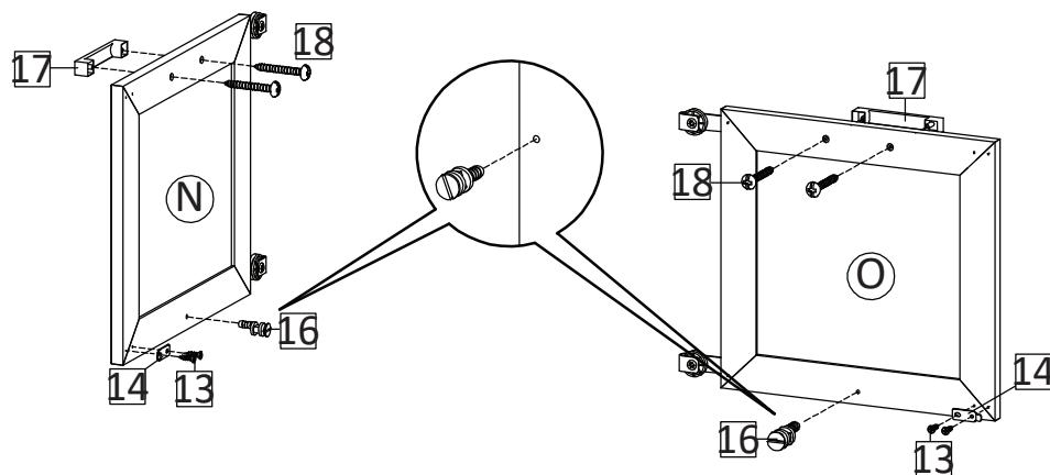
Use Screw M 3.5x25 mm (HW18) to attach Handle (HW17) to the Frame Door Left (N) and Frame Door Right (O). Also, insert Screw M 3.5x13 mm (HW13), Sliding Plate (HW14) and Stopper (HW16) as above image.
