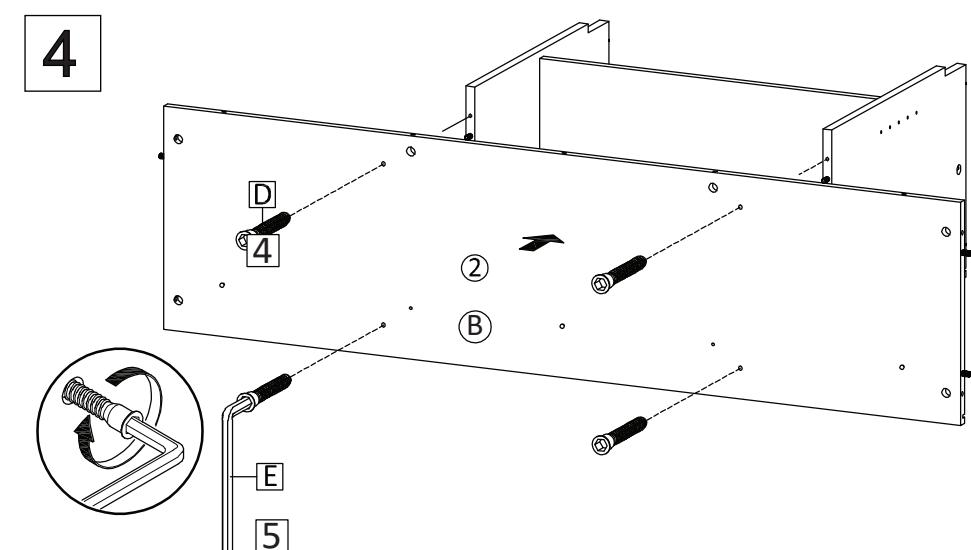
Tighten Screw M 7x50 mm (HW4) by using Allen Key (HW5) to attach Bottom Board (B) to step 3.
