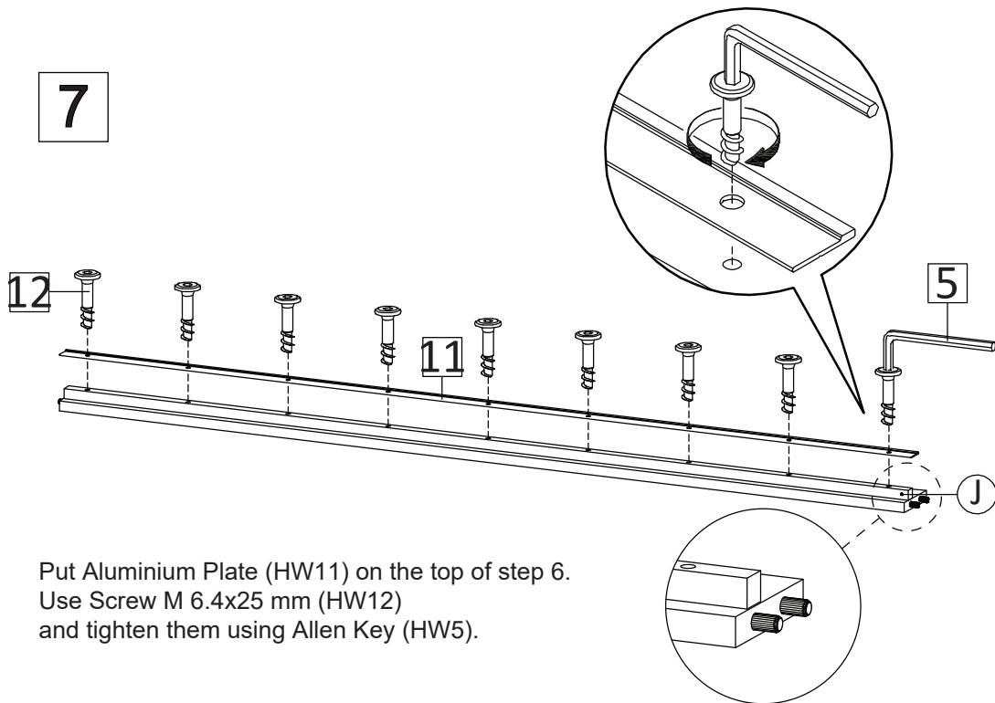
Put Aluminium Plate (HW11) on the top of step 6.
