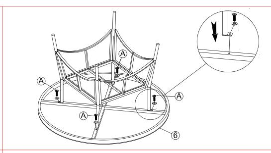
STEP 6 : Connect The Part from Step 5 and Table Top (6), tighten Bolt (A), Flat Washer (D) with Allen Key (E).
