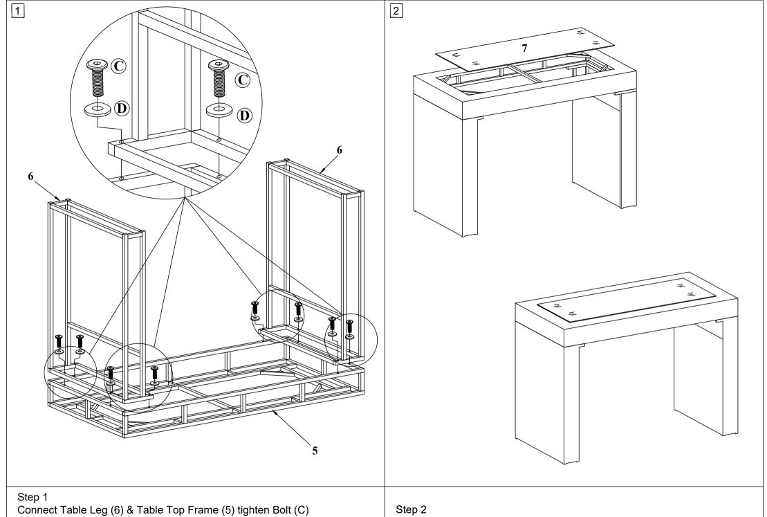
Connect Table Leg (6) & Table Top Frame (5) tighten Bolt (C) with Allen key (E)
