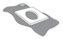
2. Position the sink over its cutout on the counter top. Make sure the sink is centered with the faucet hole and is evenly spaced between the bolt holes.
