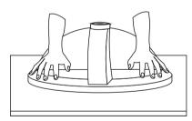
6. At each of the bolt holes in the counter top, attach sink clips by placing the long end of the bracket flat against the sink lip. Screw the wing bolts through the brackets and bolt holes and tighten.
