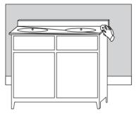
3. If you are installing a side-splash and/or back-splash, place a generous amount of silicone sealant on the back of it and press it into place against your bathroom wall. Fill any gaps that are left with silicone sealant. Wipe away any excess sealant with a damp cloth.
