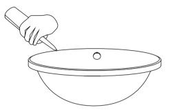
5. Carefully place the sink upside down on the counter top, positioning it within your marked outline. Once positioned, press firmly into place.
