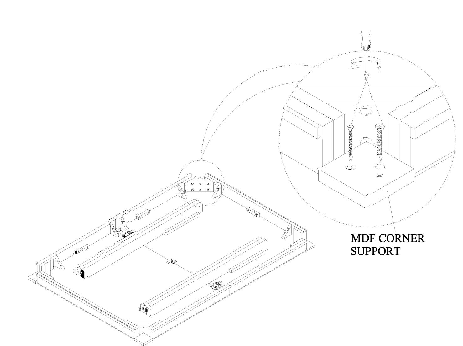
Step 1: Turn Table Top (A) upside down and put on soft surface such as carpet or cloth and then take out MDF corner support on Table Top corner by using Phillips screw driver (not included).
