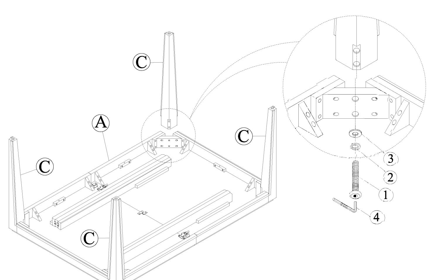
Step 2: Attach Table Legs (C) to the Table Top (A) by using Flat Washer (3), Lock Washer (2), Allen Bolt (1) and tighten with Allen Key (4).
