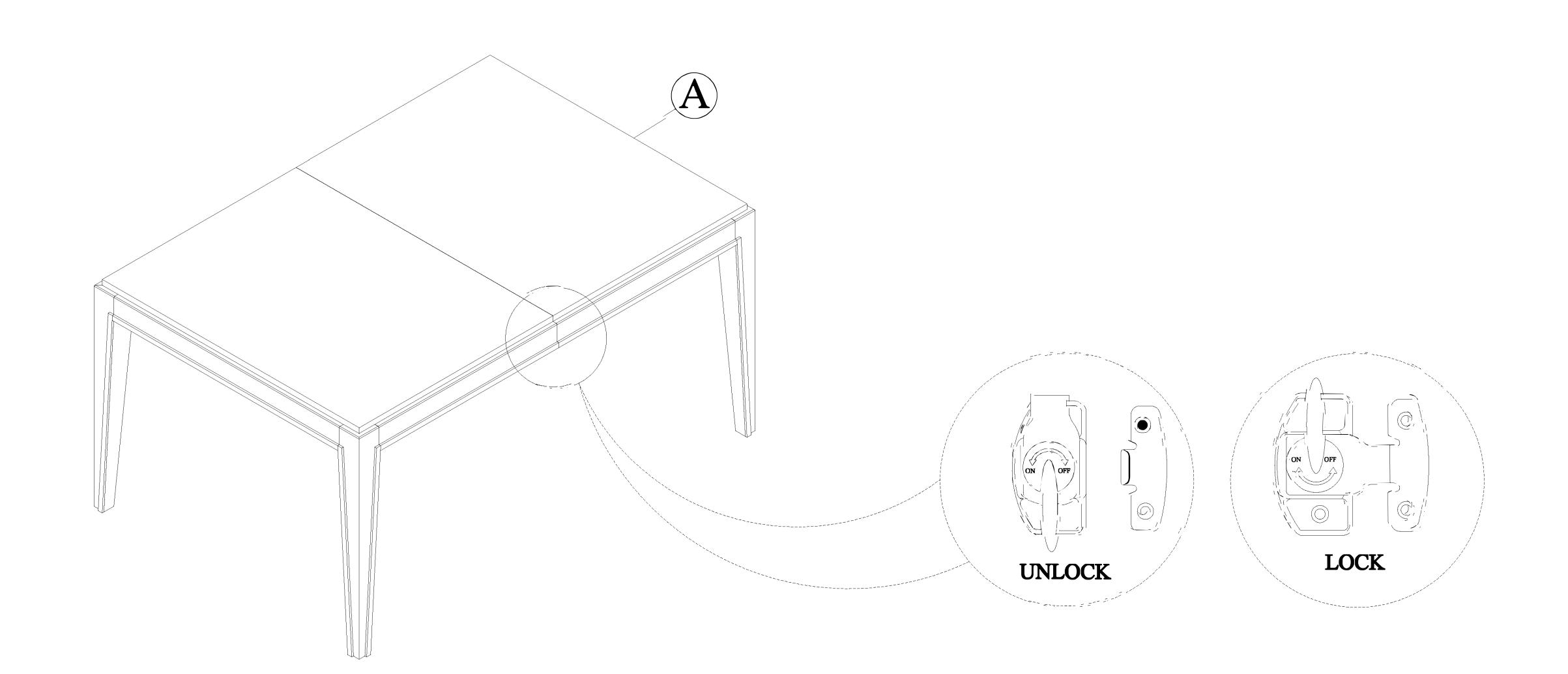
Step 3: Turn up table on upright position on level surface so that the table will not wobble and tighten all Allen Bolts by using Allen Key (4). Unlock Sash lock underneath Table Top (A).
