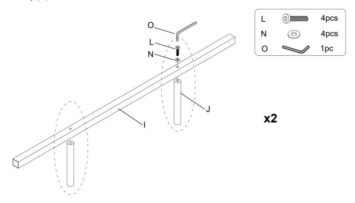
Attach Slat - Front / Rear (H) and the pre-assembled Slat - Middle (I) to Side Rail - Front (E) & Side Rail - Rear (F), using Bolt (K) & Flat Washer (N) by Allen Key (O) as below shown.
