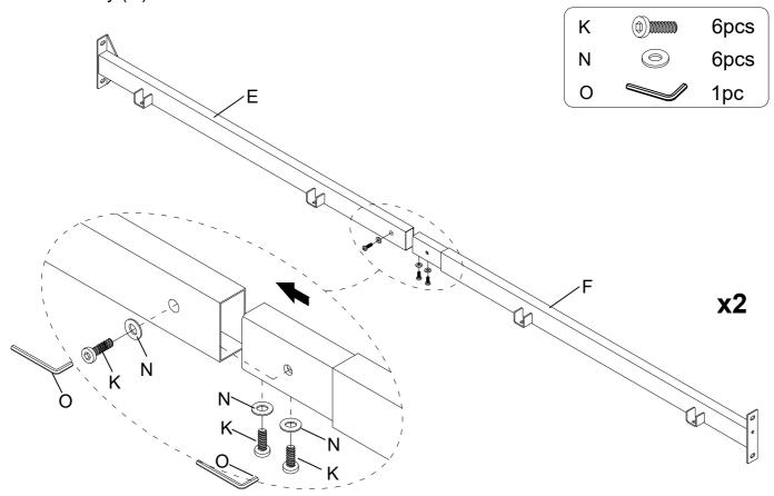
Assemble the pre-assembled Side Rail - Front (E) & Side Rail - Rear (F) to pre-assebmled Extension Leg - Left (C) & Extension Leg - Right (D) of headboard, using Bolt (M) & Flat Washer (N) by Allen Key (O), and using Nut (P) & Flat Washer (N) by Spanner (Q) to lock at the same time.
