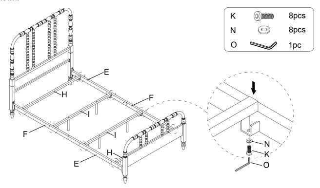
Adjust any parts out of alignment and tighten all bolts and screws from steps 1 through 6.
