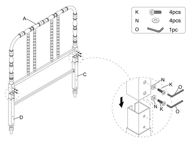
Insert Side Rail - Rear (F) to Side Rail - Front (E), using Bolt (K) & Flat Washer (N) by Allen Key (O) as below shown.
