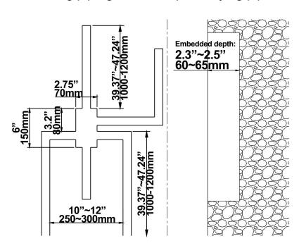
2. Install main body and inlet pipe.
