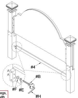
Align HB support (#4) to the HB legs, then secure by using bolts (#B) with washers (#E,F).
