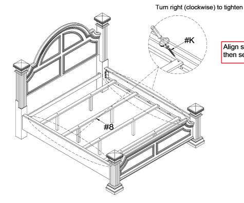
Align slats (#8) to the side rails, then secure by using screws (#K).
