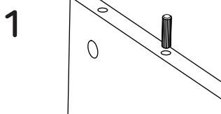
Put in the dowel inside the indicated hole and softly hit it until it's fully inside.
