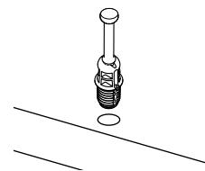
This is a spreading bolt. You should put it with the black plastic part facing down.
