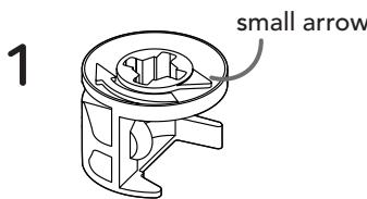
This is a Minifix cam. It has a little arrow on its upper surface.
